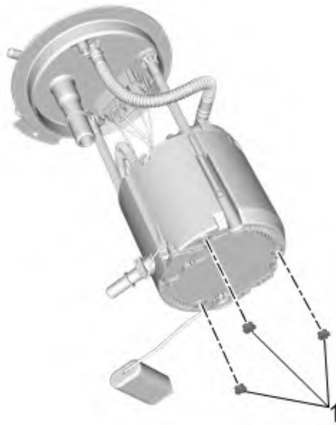
Fig. 80: Inspect Bottom Of Fuel Pump Module For Green Rubber Pads Courtesy of GENERAL MOTORS COMPANY
